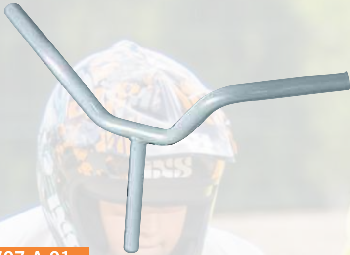
SE-707-A-01 HANDLE BAR 218 MIG/TIG WELDED DIA : 22mm THICKNESS : 1.2, 1.4, 1.6 FINISH : Raw / Black / White / CP
