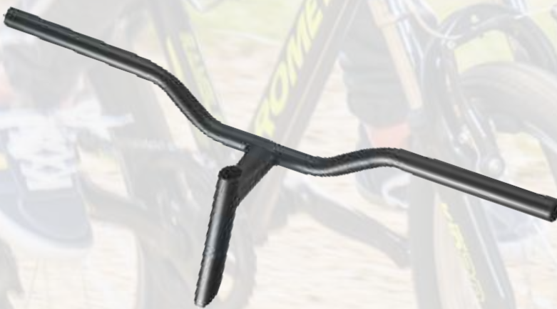
SE-707-D-02 HANDLE BAR 620x150mm MIG/TIG WELDED DIA : 22.2mm COLUMN DIA : 25mm THICKNESS : 1.2, 1.4, 1.6 FINISH : Raw / Black / White / CP
