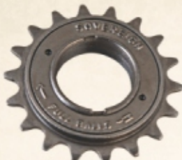
SE-2001-H-05 FREEWHEEL SINGLE SPEED Size : 1.8T (1/2x1/8) Thread Size : 34.8 x 24TPI Half Balls / Full Balls FINISH : Golden / BCP / Black / Blue
