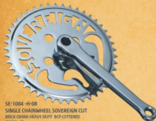
SE-1004-H-06 SINGLE CHAINWHEEL SOVEREIGN CUT EMBOSSED CRANK BCP COTTURED CRANK: 7" WHEEL: 44/46/48T THREADING: 9/16 x 20TPI L/RH FINISH: To Order
