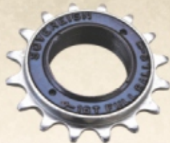
SE-2001-H-06 FREEWHEEL SINGLE SPEED Size : 2.0T (1/2x1/8) Thread Size : 34.8 x 24TPI Half Balls / Full Balls FINISH : Golden / BCP / Black / Blue
