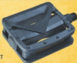
SE-376 PLASTIC HORSE SHOE MODEL body with Balls Reflector included (BS approved reflector available) Axle Thread : Optional (9/16x20TPI/ 14x1.25 / 1/2" x 20TPI) COLOUR: Black / Grey
