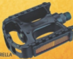
SE-378 PLASTIC HI-IMPACT body with Balls Reflector included (BS approved reflector available) Axle Thread : Optional (9/16x20TPI/ 14x1.25 / 1/2" x 20TPI) COLOUR: To Order
