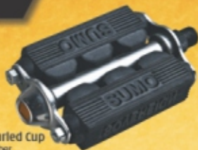
SE-382 PEDAL ANTI SKID HEAVY DUTY Reflector in Cap Axle Thread : Optional (9/16x20TPI/ 14x1.25 / 1/2" x 20TPI)
